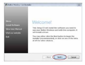
**Note:** If the Belkin Wireless Adapter Installer screen does not appear within 20 seconds, access your CD-ROM by double-clicking on the "My Computer" icon; then double-click on the CD-ROM drive into which the installation CD has been placed. Then, double-click on the icon named "Installer.exe".
